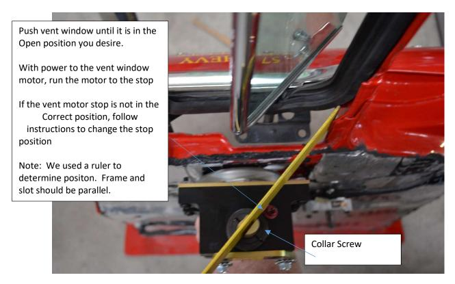
3. Once the stop is set, you can slide the power vent up on the vent window stem.
