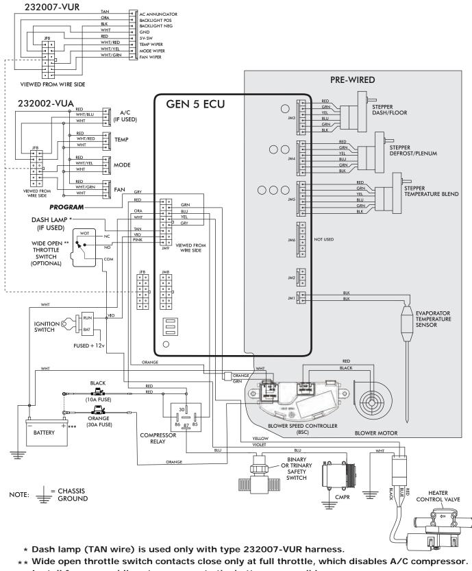
\*\*\* Install fuse assemblies at or as near to the battery as possible.
