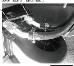
Install 90° fitting on #6 drier/evaporator A/C hose onto block valve adapter
