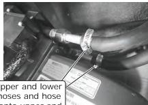
Install upper and lower heater hoses and hose clamps onto upper and lower heater hardlines
