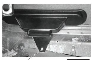
Install passenger-side defrost duct using #12 x 1/2" self-tapping screw
