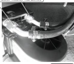
Install 90° fitting on #6 drier/evaporator A/C hose onto block valve adapter
