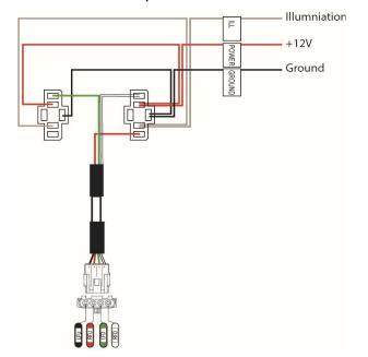
**Illumination (Gray)** - This wire provides power to the switch lights. It should be hooked up to a light circuit in the vehicle (dash lights) or it can be hooked up to a 12 volt switched source.
