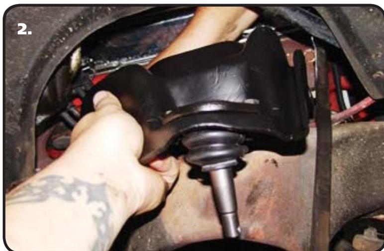
**2.** Insert the Balljoint into the Control Arm from the top side of the Control Arm with the Balljoint Pin Sticking down. Attach it to the Control Arm with the Hardware Supplied with the Balljoint. Torque the Hardware to 14 ftlbs. Engage the Balljoint Pin into the Spindle and install the Castle Nut Supplied. Torque the Castle Nut to 50 ftlbs and tighten to align Cotter Pin Hole. Install Cotter Pin through Hole and Bend Pins to prevent falling out.
