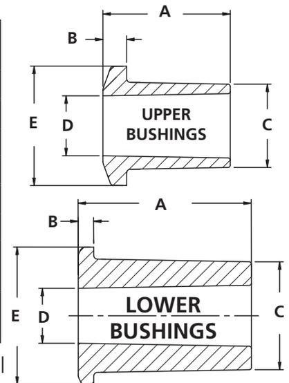
The 73-74 has 2 possibilities for the Front Bushing of the Lower Control Arm. The 2 possibilities are in **BOLD** in the chart.
