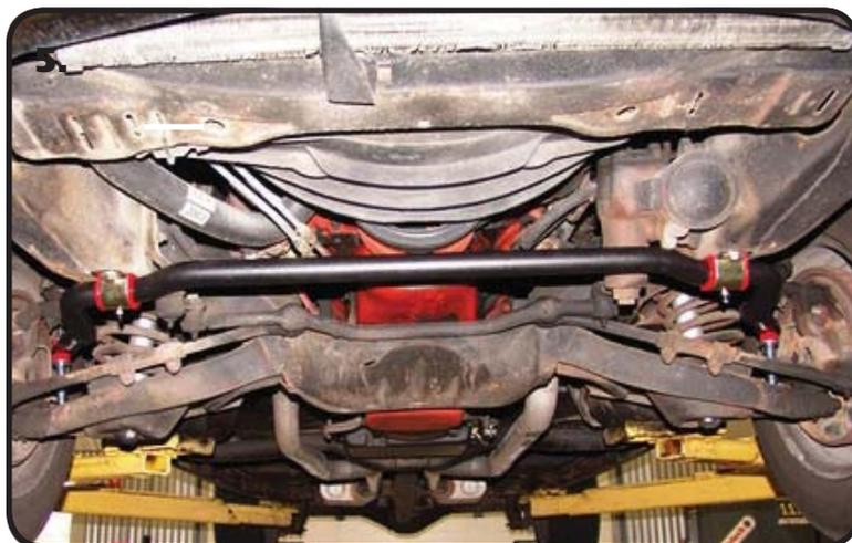
5. Slide the SwayBar into position on the Car. The SwayBar Arms will be above the Tie Rods. Slide the Front Hole of the SwayBar Bushing onto the 3/8" -16 Stud. Hold it in place with a 3/8" SAE Flatwasher and 3/8" -16 Nylok Nut. Install the Correct Lockwasher and Flatwasher on the Correct Hex Bolt. Do **NOT** Complete tighten the Hardware. It will be left partially loose until the End Links are installed.
