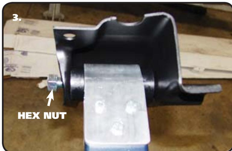
3. Bolt the **LARGE BUSHING END** of the Composite Leaf Spring into the OEM front leaf spring mount using a 1/2"-13 x 5" Hex Bolt and 1/2"-13 Nylok Nut. The Bolt must be installed with the threads pointing to the **OUT-SIDE** of the car. Diagram #4 is the correct.
