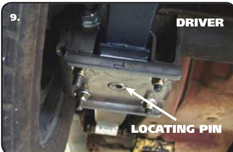
**9.** Lower the differential onto the Leaf Spring with the top Clamping Plate in place like shown in Diagram "6". The TAB on the Top Clamping Plate will nest in the NEW leaf spring mount. Install the lower Clamping Plate followed by the NEW lower mount **being sure the Pins and Holes are aligned**. Install the OEM hardware.
