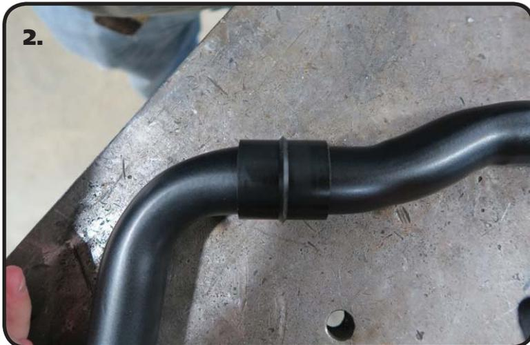
**2.** The Delrin Liner is split on one side to ease installation. We found it easier to install by opening up the Liner enough to slide it onto the end of the SwayBar, then sliding it into position. It will open up and slide over the curves in the Bar. Install a Liner on each side of the SwayBar in the approximate location they will need to be when installing the SwayBar on the Car.
