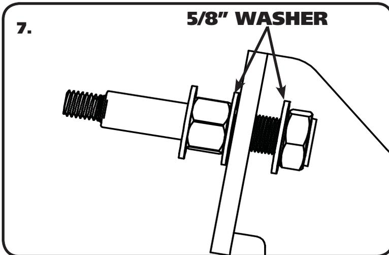
**7.** We recommend installing the Shock Studs in the Leaf Spring Clamping Plate before installing the plates in the car. The Shock Studs are supplied in the kit. Refer to **Images 7-9** for proper installation. The shock stud hardware is packaged with the stud. Install a 5/8" washer onto the 5/8" threads. Insert the stud into the hole on the plate. Install a washer on the threads, followed by a 5/8"-18 Locknut. Tighten 5/8" Nut.
