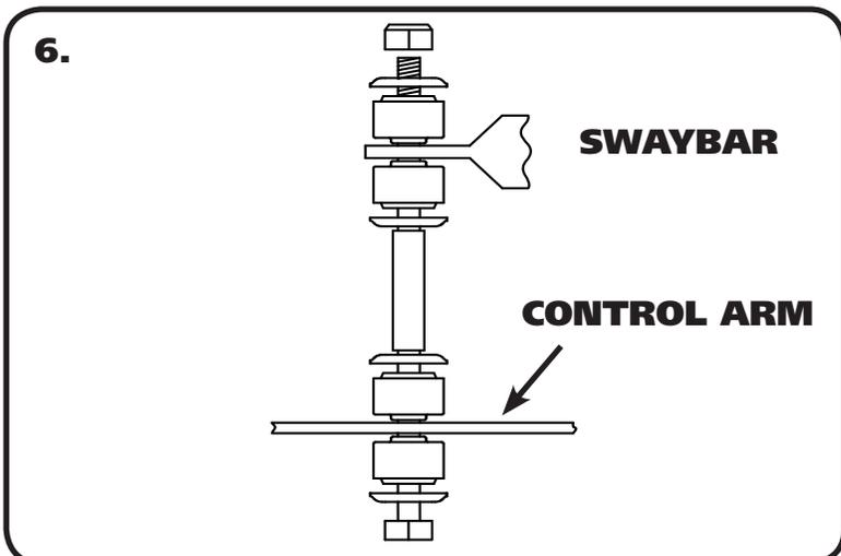
6. Install the End Links. Use Diagram "6" for proper installation. Tighten the Hex Nut enough to slightly compress the Bushings.
