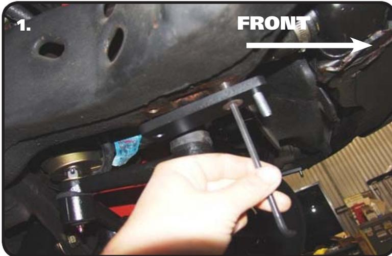
**1.** Attach the Adapter Plate to Frame positioned with the 3/8"-16 Stud to the Front of the Car and the Rear Hole aligned with the Rear OEM Hole. The Adapter Plate is attached to the Frame using a Flat Head Bolt and Red Loctite. The OEM Threaded holes can be either, 5/16"-18 or 3/8" -16, hardware is supplied for each. Apply Red Loctite to the proper Bolt and insert it through the Adapter. Thread the Bolt into the Front OEM Hole and tighten.
