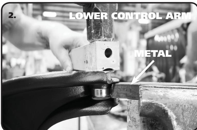
2. Disassemble the Bushing being installed. If installing Bushings in the Upper Control Arm, insert the Cross Shaft before installing any Bushings. Support the Back Side of the Flange the Bushing is being Installed in. Use a STIFF piece of Metal clamped in a Bench Vise for the Lower Control Arms (**Figure 2**). The Upper Control Arm can be supported by either the same piece of Metal or by the Bench Vise with the Jaws opened wide enough to let the Bushing Shell pass through (**Figure 3**).
