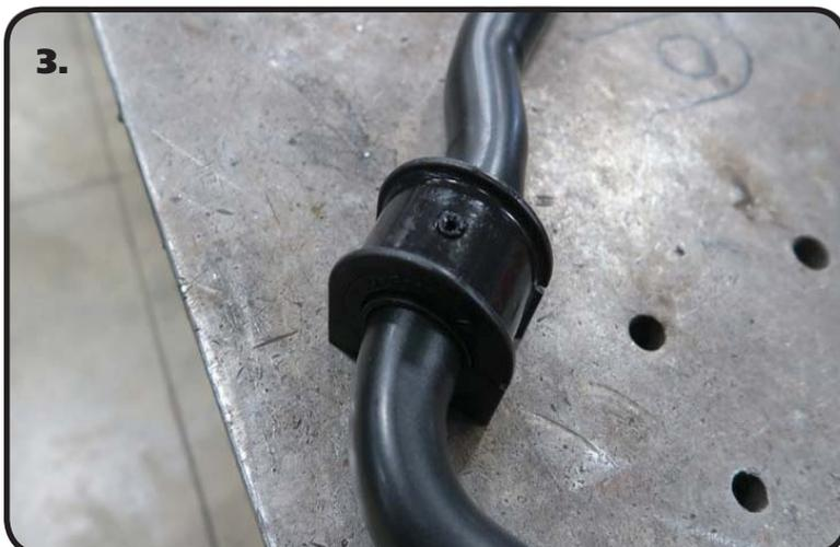
**3.** Open up the Poly SwayBar Bushings and install them over the Delrin Sleeves.
