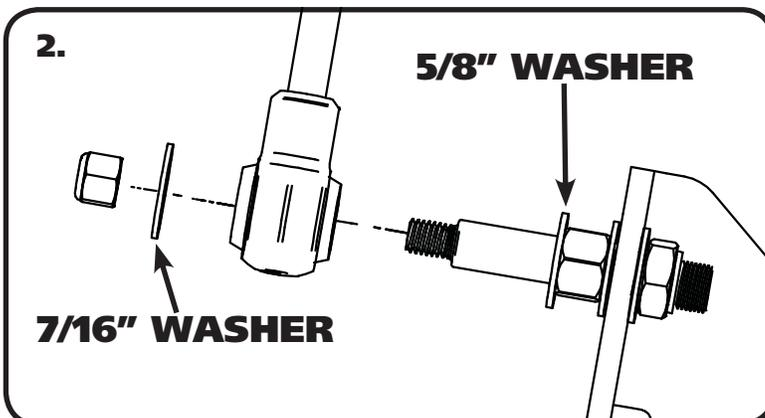
2. Install a 5/8" washer on the shock stud. Slide the shock onto the stud. It may be necessary to raise the differential to get the shock on the stud. With the shock on the stud, install a 7/16" Flatwasher followed with a 7/16"-20 nylok nut. Tighten nylok nut.
