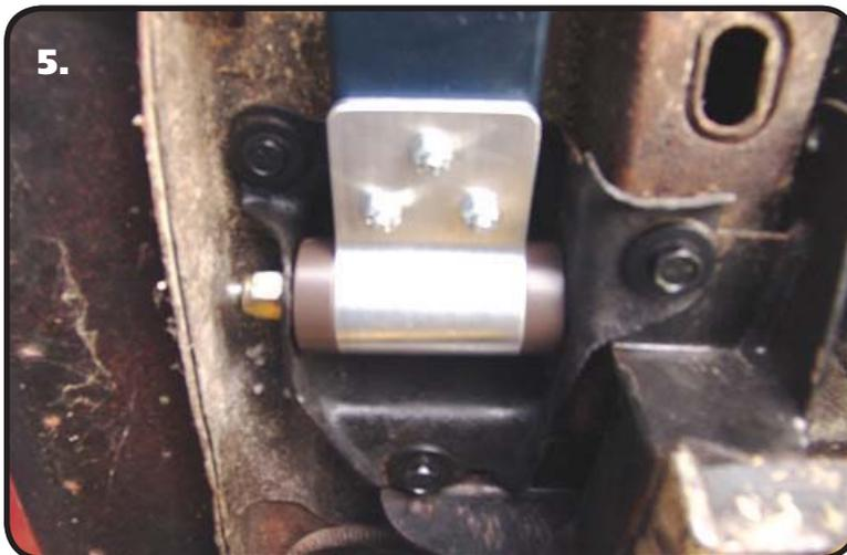
5. Swing the Leaf Spring up and attached the front mount to the car using the supplied 3/8"-16 x 1 1/2" Conical Body Bolts and U-Nuts. Tighten Hardware
