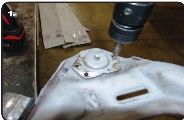
**1.** If your Balljoints are Bolted to the Control Arms, simply unbolt them. If your car has the Original Balljoints, they will be Riveted to the Control Arms. The Rivets can be removed by Grinding the Heads off and driving them out with a Hammer and Punch.
