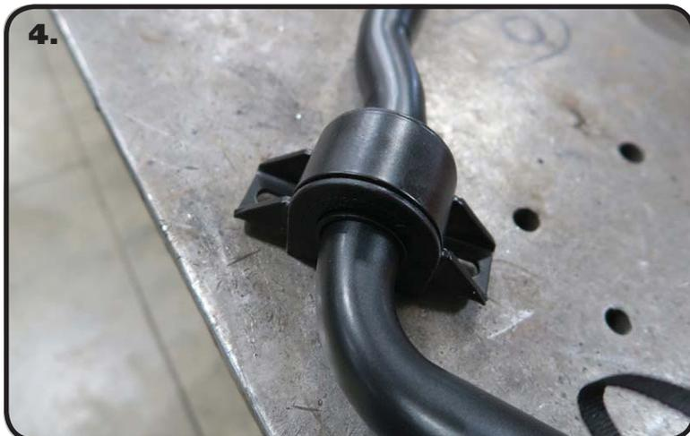
4. Install Bushing Straps Over the Poly SwayBar Bushings.
