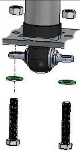
2. Attach the Trunnion to the OEM Control arm using the supplied 5/16" Hardware. Install a 5/16" Lock Washer followed by a 5/16" Flat Washer on each of (4) 5/16"-18 x 1" Hex Bolts. This Hardware will be inserted into the holes in the Shock Trunnion to attach the shocks in the OEM Location. It may be necessary to rotate the Trunnion to get it in the correct position. This can be done by sticking a screwdriver in one of the slots and spinning the trunnion in the shock bushing.
