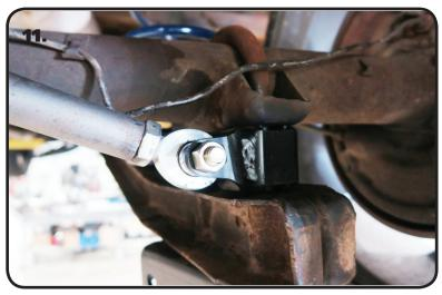
**11.** Repeat the procedure in step 9 on the axle side of the Panhard Bar. You may need to push the rear differential to one side or the other to get the Panhard bar lined up in the Mount.
