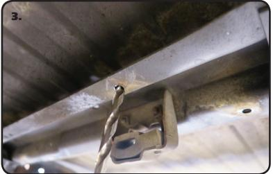
3. Drill the 4 rivet holes out to 7/16".
