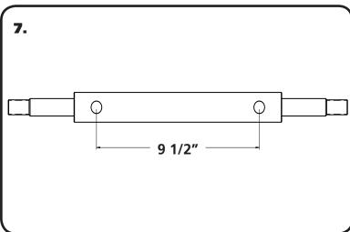
**7.** The Lower Cross Shaft has 2 different locating Hole patterns. This StreetGrip kit uses the 9 1/2" center to center locating holes. The Pin in the Cross Shaft Saddle will locate into these Holes.
