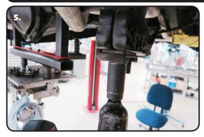
**5.** Remove the OEM lower shock mount by removing the u-bolt nuts. Remove the U-Bolts.
