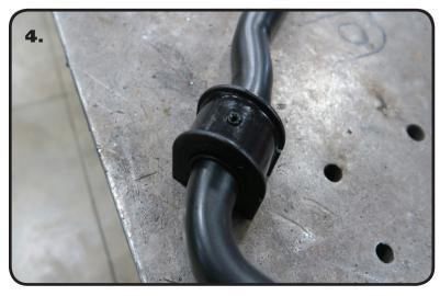
**4.** Open up the Poly SwayBar Bushings and install them over the Delrin Sleeves.
