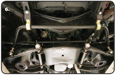
**6.** Hold the SwayBar into position on the truck with the SwayBar arms below the tie rods. Align the holes in the Bushing Straps with the holes in the Frame Brackets. Install a 3/8" Flat Washer on (4) 3/8"-16 x 1 1/4" Hex Bolts and insert them into the holes. Install a 3/8" Flat Washer and 3/8"-16 Nylok Nut on each Bolt. Center the bar in the bushings before snugging up the hardware. Do **NOT** completely tighten the Hardware. It will be left partially loose until the End Links are installed.
