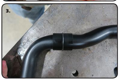
If your truck is equipped with an OEM Swaybar, remove it to prepare for the StreetGrip SwayBar installation.
