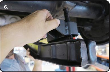
**6.** The kit contains 2 spacer blocks with one having the panhard mount welded to it. The spacers are installed between the axle and the trailing arm. The spacer block with the mount welded to it is installed on the passenger side with the mount positioned to the rear inside. Remove the OEM u-bolt and install the u-bolt supplied in the kit. Slide the spacer block onto the u-bolt followed by the OEM trailing arm.
