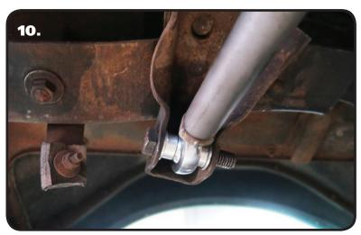
**10.** Install the panhard bar in the frame mount. Install a 5/8" Flat Washer on a 5/8"-18 x 3 1/2" Hex Bolt and insert it through the Mount, Spacers and Panhard bar. With the Bolt installed, install a 5/8" Flat Washer on the threads followed by a 5/8"-18 Nylok Nut.
