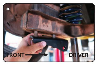
**8.** Next, install the Lower Shock Brackets. The brackets are installed on the U-Bolts, on the bottom side of the trailing arm. The shock mounting hole should be positioned with the hole to the front and to the inside of the truck. Once the Mount is installed, install a 3/4" Flat Washer and 3/4"-16 Nylok Nut on each leg of the U-Bolts. Tighten the Nylok Nuts to 350ftlbs.
