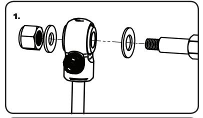
1. The Shock is supplied with 5/8" & 1/2" Sleeves. If the Sleeves are not installed, insert a 5/8" Sleeve in the shock eyelet bushing and the 1/2" Sleeve in the shock body bushing. They can be pressed in with a bench vise. Install the Eyelet of the shock on the OEM frame stud using the OEM hardware. Position the Shock with the Adjuster Knob pointing out, away from the frame.
