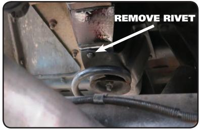
1. The Rivet needs to be removed from the rear of the OEM coilspring mount. One way is to cut a "+" in the head of the rivet and chisel the 4 pieces of the head off the rivet, then knock the rivet out of the frame with a hammer and punch. It can also be drilled out.
