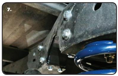
7. Install a 7/16" Flat Washer on (5) 7/16"-14 x 1 1/4" Hex Bolts. Insert them through the holes in the frame side. Install a 7/16" Flat Washer and 7/16"-14 Nylok. Install a 3/8" Flat Washer on (4) 3/8"-16 x 1 1/4" Hex Bolts, insert them in the bottom holes and install a 3/8" Flat Washer and 3/8"-16 Nylok Nut on the threads sticking through. Tighten all hardware and repeat on other side.
