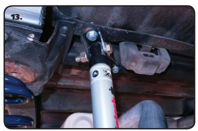
**13.** The Shock is mounted in the Upper Mount with the BODY UP. It is held in place with a 1/2"-20 x 2 3/4" Hex Bolt & 1/2"-20 Nylok with a 1/2" Flat Washer on each side of the bracket.
