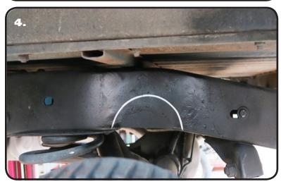
**4.** Diagram "3" shows the frame rail marked before cutting. The bottom of the frame will also need marked for cutting.
