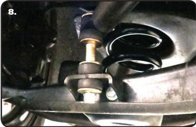
**8.** Install a 3/8" Flat Washer on (2) 3/8"-16 x 1 1/4" Hex Bolts and insert them into the holes. Install a 3/8" Flat Washer and 3/8"-16 Nylok Nut on each Bolt. Repeat on the other side and tighten hardware.
