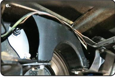
**6.** Slide the C-Notch into the frame rail.
