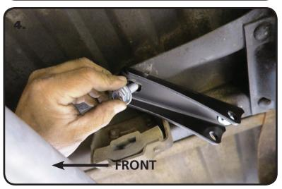
**4.** Install a 7/16" Flat Washer on each 7/16"-14 x 1 1/4" Bolts. Position the Shock Bracket in the same location as the OEM shock mount with the shock mounting holes to the rear of the truck. Line up the front and rear holes and insert the 7/16" Bolt/Washer from the bottom with the threads pointing up. Install a 7/16" Flat Washer and 7/16"-14 Nylok on the threads of the bolt. Repeat steps 3-5 on both shock mounts. Tighten Hardware.
