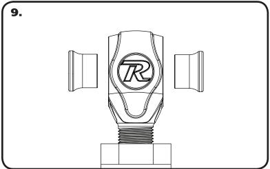
**9.** Install the R-joint Spacers into the center pivot ball of the R-Joint. Insert the small end of the spacer into the center ball, push it in until it stops.
