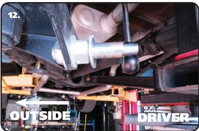
**12.** Install the supplied Shock stud in the Lower Shock Mount. The stud should be installed with the STUD pointing to the center of the truck. Install a 5/8" Washer (supplied with stud kit) on the 5/8"-18 Thread side of the Stud and insert it into the Shock Bracket. Install a 5/8" Washer and Nylok Nut on the threads and tighten. Do this for both shock brackets, installing the Studs with the small threads pointing to the center of the truck.
