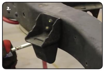
**2.** Remove the OEM bumpstop mounts from the frame rails by removing the rivets. Again, one way is to cut a " +in the head of the rivet and chisel the 4 pieces of the head off the rivet, then knock the rivet out of the frame with a hammer and punch. It can also be drilled out.
