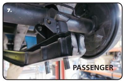
**7.** Diagram "5" shows the passenger spacer block installed. Note the position of the panhard mounting tabs.
