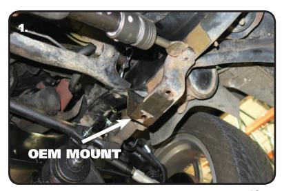
1. Some trucks are equipped with a OEM swaybar. If your truck has one, the OEM mount will need to be removed to install the MuscleBar. This is done by removing the rivets. The rivets can be removed by chiseling the heads off and driving them out or by drilling the rivets out. The new Frame Mount bolts directly in place of the old mount. If your truck doesn't have a sway bar, the mounting holes will still be in the frame.
