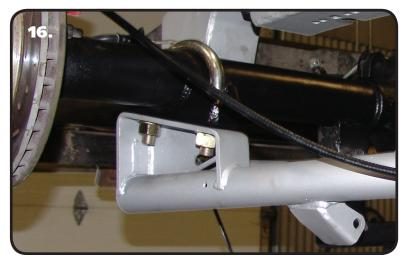
**16.** Bolt the other end of the StrongArm to the axle using the new U-bolts supplied.
