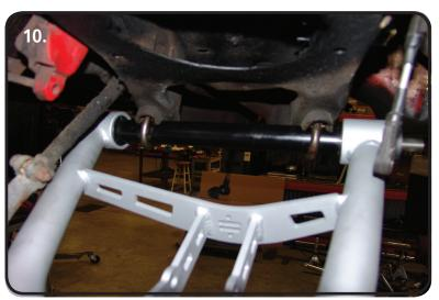
**10. Image 10** is an example of the lower bolted to the crossmember. Install 3/4" ID Washer on to each end of the crossshaft against the bushing. Then install the 3/4"-16 lock nut. Snug the nut up against the washer. You want the suspension move freely through its travel.
