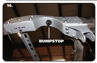
**14.** Install the bumpstops into the "C" Notch using a 3/8" nut and flatwasher.
