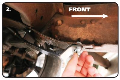
2. The MuscleBar Mount attaches to the frame using the holes from the OEM mount. The end of the frame bracket with the angled bends goes forward. Attach the bracket using a 3/8"-16 x 1 1/4" bolt, 3/8"-16 Nylok nut and a 3/8" Flat Washer on top and bottom. The same hardware setup is used in each hole. Repeat on the other side and tighten hardware.
