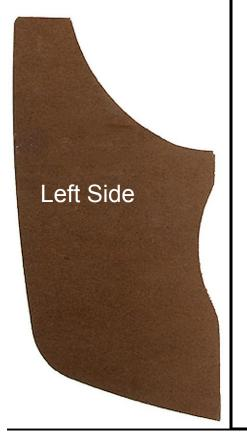
These are the next panels to go into the trunk. Put the left side in by matching the cutout with the hump near the bottom of the wheel well tub. Be careful not to break the panel by forcing the piece into place. Start by sliding the front of the panel under the edge of the trunk fender then slide the cutout into place. The panels should fit under the edge of the trunk lip. The side panels should be on top of the floor panel on both sides.
