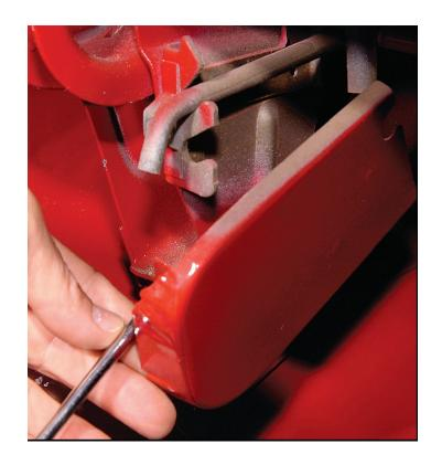
This is a picture of the bottom floor panel for the 55, 56, 57 Chevy. The panel is big and needs to be placed in the trunk tilted right side down and in first. Set the panel on the floor of the trunk then slide it back toward the trunk latch. The tail light wires should be moved out of the way or wire tied up in order to seat the panel properly in the trunk.
