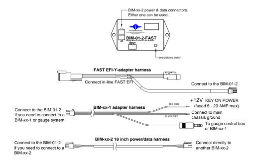
This Bus Interface Module is designed to read engine information from FAST XFI and TCI EZ-TCU kits. FAST EZ-EFI kits are <u>not</u> compatible. This module is connected to the FAST/TCI kits through the included Y-adapter harness. This can be plugged in line with the dedicated CAN terminals on the EFI/TCU harness.
