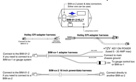
This Bus Interface Module is designed to read engine information from specific Holley EFI kits. These kits include Holley Terminator, HP, Sniper and Dominator. The module is connected to the Holley EFI through the CAN-bus plug on the EFI harness. Depending on your EFI module you may have a 2-pin or 4-pin CAN connector. We supply EFI adapter harnesses that will allow you to connect with your particular kit.
