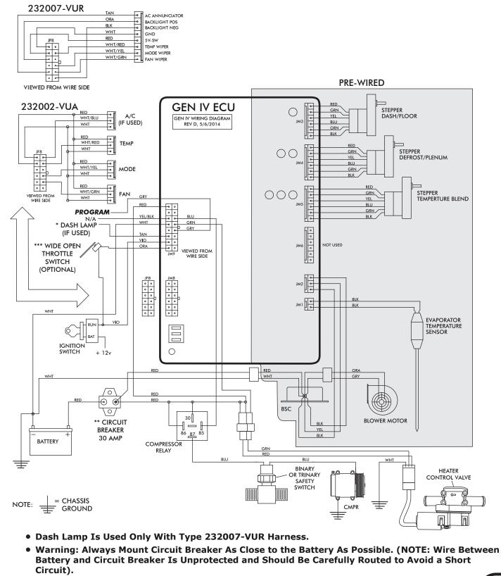
• Wide Open Throttle Switch Contacts Close Only at Full Throttle, Which Disables A/C Compressor.
