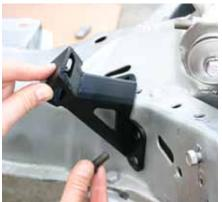
4. Using the new mounts as a guide drill four holes 3/8" through the top of the crossmember. Install the remaining bolts through these new holes, again the nuts will be on the inside of the crossmember.
