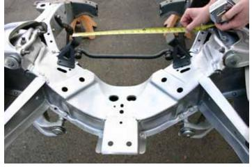
3. Position the new mounts on the crossmember so they are straight and evenly spaced. Tighten the mounts to the frame.
