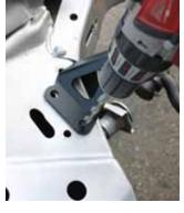
2. Using the empty rivet holes loosely attach the new engine mounts to the cross member. You will need to install two bolts into each mount through the slotted holes in the new mounts and into the frame: the nuts will be installed on the inside of the front crossmember.
