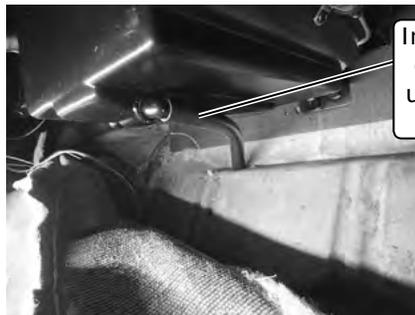
Install drain hose onto outlet on evaporator unit and through 5/8" hole on firewall
