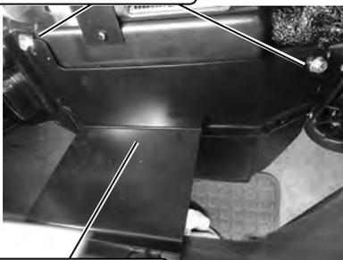
Place Evaporator Dash Bracket into Position Between Evaporator and Dash
