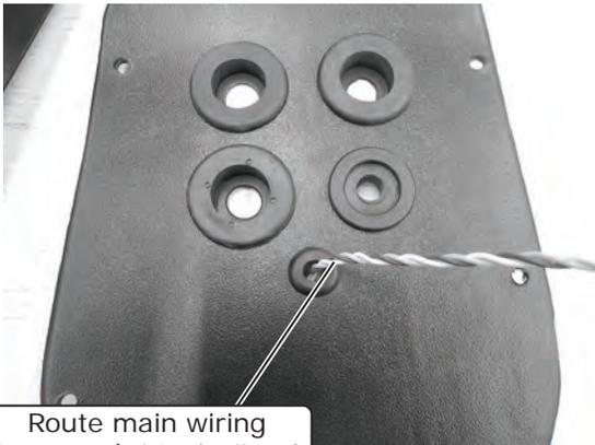
Route main wiring harness (white/yellow/purple) through 7/8" wiring grommet on kick panel fresh air cap
