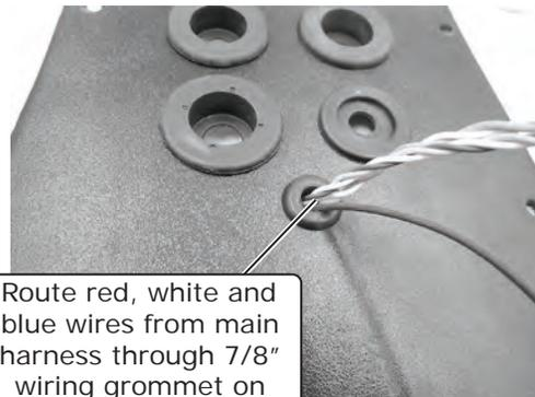
Route red, white and blue wires from main harness through 7/8" wiring grommet on kick panel fresh air cap
