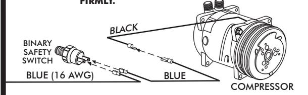
**NOTE: CONNECT WHITE WIRES DIRECTLY TO (-) BATTERY TERMINAL**
