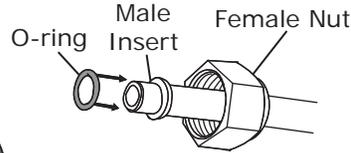
For a proper seal of fittings: Install supplied O-rings as shown and lubricate with refrigerant oil.
