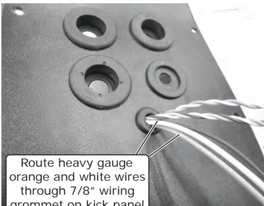
Route heavy gauge orange and white wires through 7/8" wiring grommet on kick panel fresh air cap
