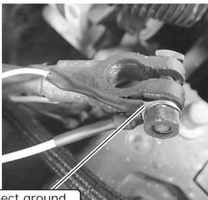
Connect ground wiring eyelets to negative battery terminal connector
