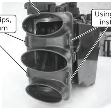
Using (2) spring clips, install dash plenum
