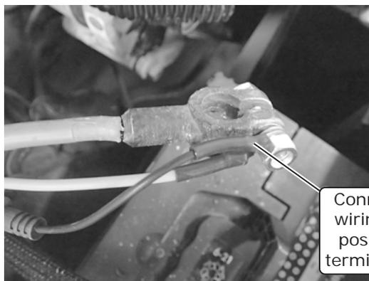
Connect positive wiring eyelets to positive battery terminal connector
