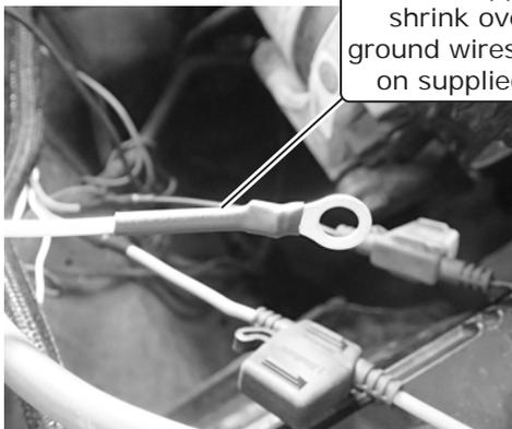
Install supplied heat shrink over white ground wires and crimp on supplied eyelets
