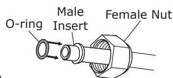
**For a proper seal of fittings: Install supplied O-rings as shown, and lubricate with supplied oil.**
