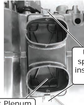
Using (2) spring clips, install defrost plenum
