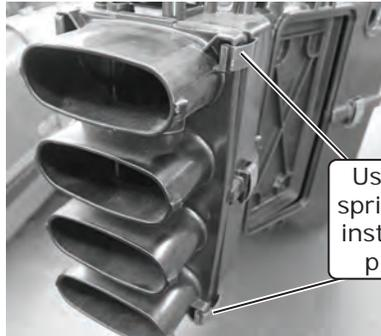
Using (2) spring clips, install dash plenum
