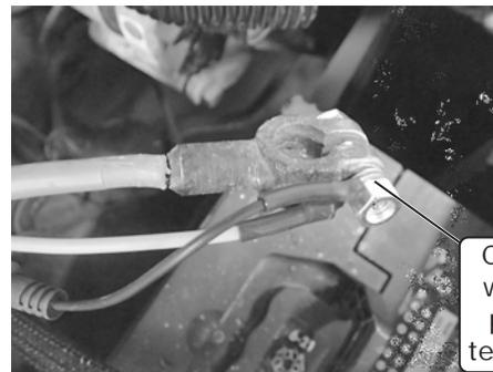
Connect positive wiring eyelets to positive battery terminal connector
