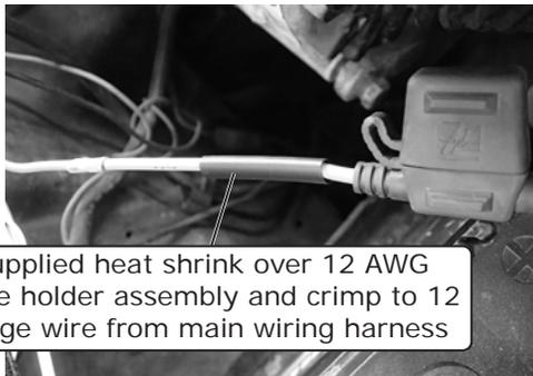
Install supplied heat shrink over 12 AWG orange fuse holder assembly and crimp to 12 AWG orange wire from main wiring harness
