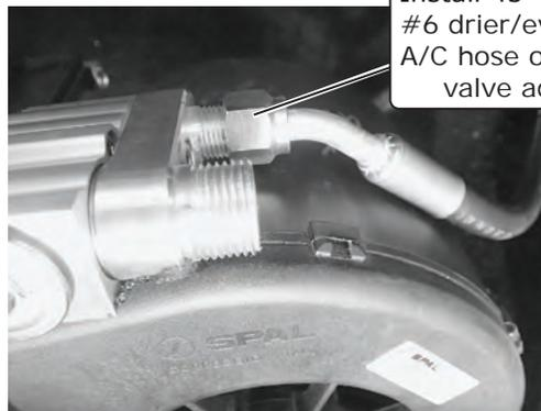
Install 45° fitting on #6 drier/evaporator A/C hose onto block valve adapter
