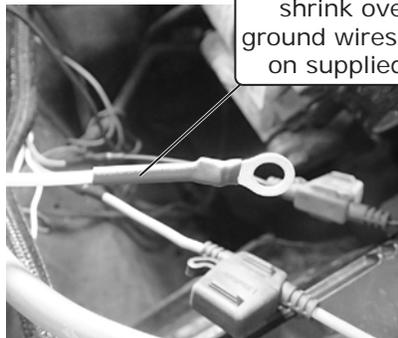
Install supplied heat shrink over white ground wires and crimp on supplied eyelets
