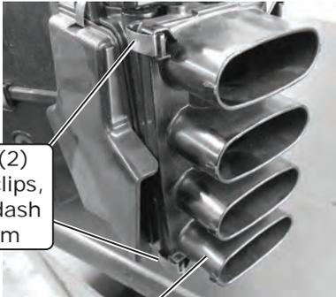
Using (2) spring clips, install dash plenum
