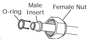
For a proper seal of fittings: Install supplied O-rings as shown and lubricate with refrigerant oil.
