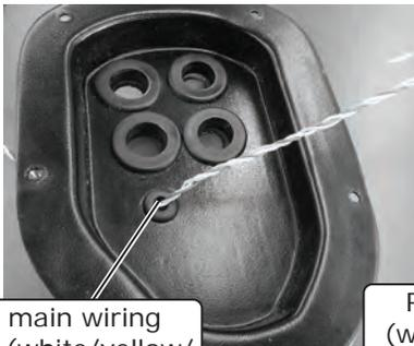
Route main wiring harness (white/yellow/purple) through 7/8" wiring grommet on kick panel cover
