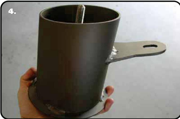
4. Thread the 6" stud into the nut in the bottom of the cup.
