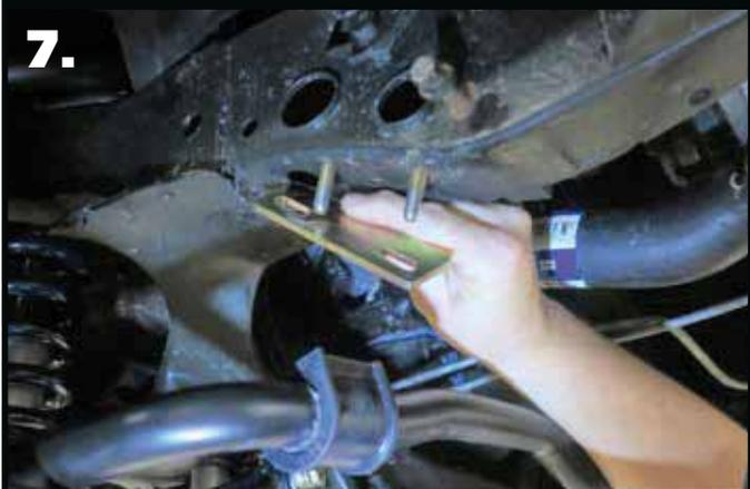
**7.** Install a 5/16" flat washer on each of (2) 5/16"-18 x 1 1/4" bolts and insert them into the OEM sway bar holes by inserting them in through the access holes in the side of the frame. Install the spacer plate with the wide side positioned to the inside. Hold it in place.
