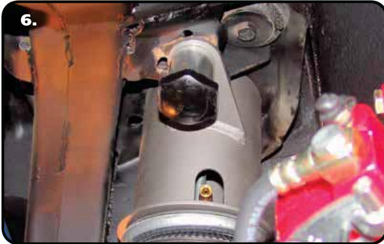
**6.** Fasten the aluminum bump stop spacer to the frame using a 3/8" x 1" bolt, flat washer and lock washer. Torque to 15 ft-lbs. Screw the bump stop into the spacer.
