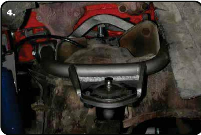
4. The Upper Control Arm is attaching the factory mount using factory hardware. Reinstall the shims in the location they were removed from. The passenger side arm is shown in **Figure "4"**. Torque the OEM nuts to 50 ft-lbs.
