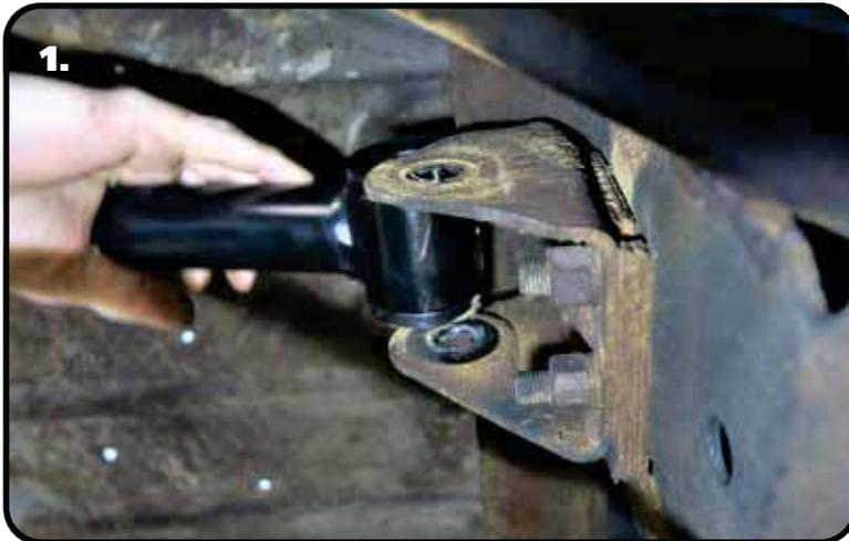
**1.** Insert the Bushing end of the Upper Control Arm into the OEM mount. The control arm should be installed with the bend upward for better axle clearance. Install a 5/8" flat washer on a 5/8"-18 x 3 3/4" hex bolt through the mount and control arm bushing. Install a 5/8" flat washer, followed by a 5/8"-18 nylok jam nut onto the threads of the bolt. Tighten the hardware enough to eliminate any gaps.
