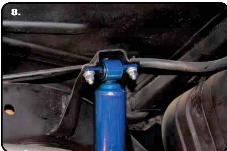
**8.** Attach shock T-Bar to frame using 5/16" x 1" bolts, Nylok nuts and flat washers. Torque to 17 ft-lbs.
