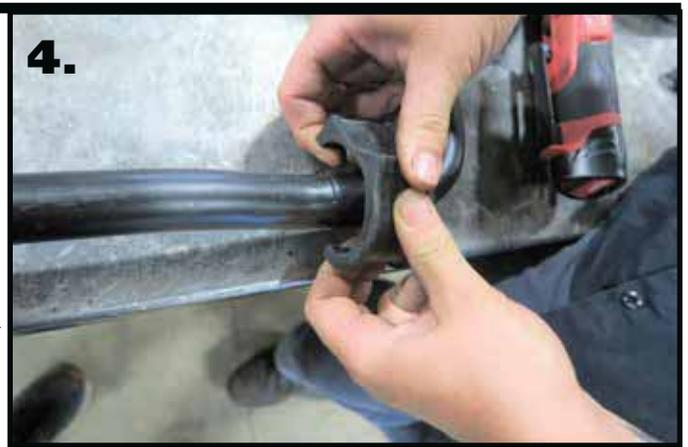
**4.** Open the sway bar bushing at the split and slip it **OVER** the sway bar. Do this for both bushings
