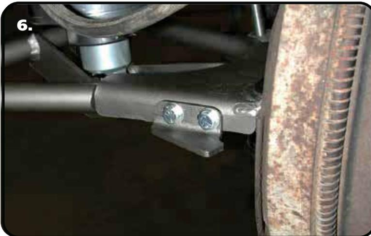
6. Attach the adjustable steering stop to the lower arm using (2) 5/16" x 1" bolts, (4) 5/16" flat washers, & (2) 5/16"-18 nylok nuts.. This can be adjusted to maintain tire/shock clearances. Torque the steering stop hardware to 25 ftlbs.
