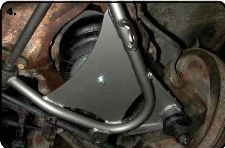
4. Attach the shock to the lower control arm, refer to the shock kit instructions. Also, attach the airspring to the lower control arm using the hardware supplied with the CoolRide kit.
