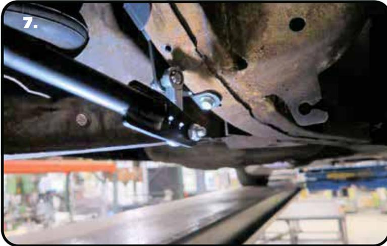
7. Install the PosiLinks in the frame brackets and in the FRONT hole in the MuscleBar. **The Posilinks are installed with the stud on the upper PosiLink pointing outward and the stud on the lower PosiLink pointing to the inside of the car.** Install the 10mm Nylok on Posilink and tighten nut.
