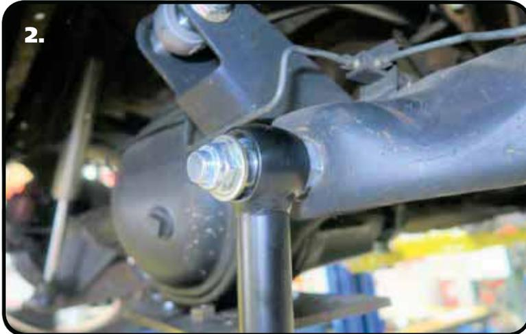
2. Install a Narrow 5/8" ID R-joint Spacer into the R-joint. The Small Diameter goes into the R-joint. Slide the R-joint onto the stud and fasten in place with a 5/8" flat washer and 5/8"-18 thin jam nylok nut. Torque to 95 ftlbs.
