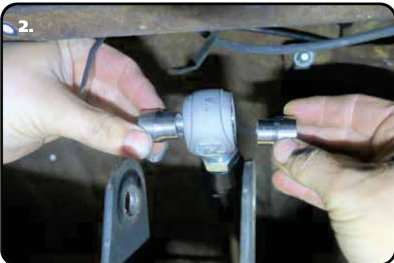
**2.** Insert the small diameter of the R-Joint Spacers into the center ball of the R-Joint. Insert the R-Joint/Spacers into the OEM mount of the differential.
