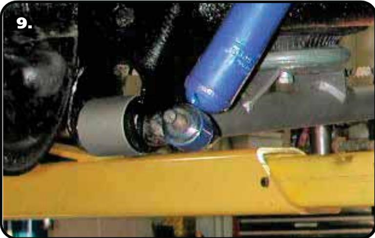
9. Attach the bottom of the shock to factory shock stud using the 1/2" Nylok nut & flat washer supplied. Torque to 45 ft-lbs.
