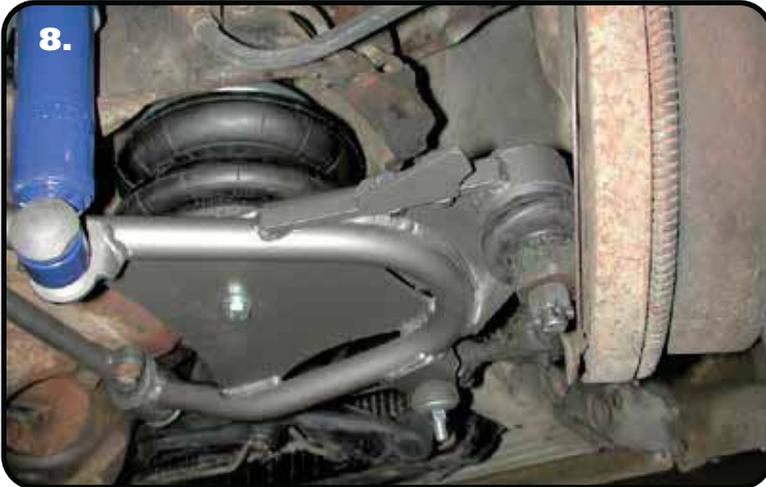
**8.** The air spring will be attached to the lower arm using a 3/8" x 3/4" bolt, lock washer and flat washer. Torque the 3/8" bolt 15-20 ft-lbs.
