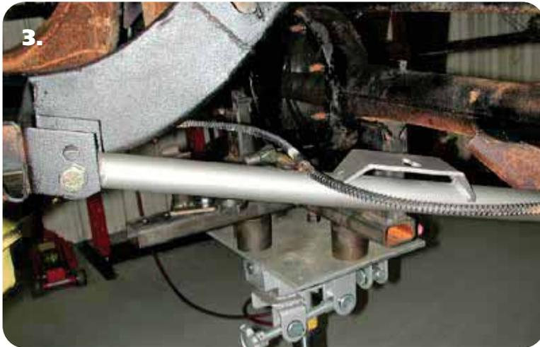
3. Fasten the front of the lower StrongArms to the frame using the 5/8" x 3 3/4" bolts, flat washers, and nylok nuts supplied. The OEM rear bolt will be reused in conjunction with the supplied flat washer and Nylok nut. Tighten the bolts/nuts enough to eliminate any gaps.
