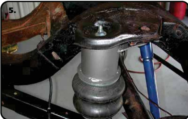
5. Place the air spring assembly into the coil spring pocket with the tab on the side of the cup aligning with the factory bump stop mount. The stud should poke through the hole in the upper coil spring pocket. Some cars may not have this hole and it must be drilled with a 7/16" drill bit. Fasten with a 7/16" Nylok nut and flat washer.
