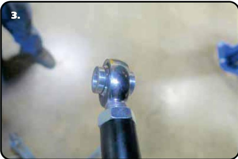
3. Install the 3/4" jam nut onto the end of the Heim end, then screw Heim end into the end of the panhard bar. Set the Panhard Bar to 31.500". You may need to readjust it after getting the car set at ride height, but this is a good starting point. Press the SMALL diameter of the aluminum 9/16" ID T-bushings into the Heim end.
