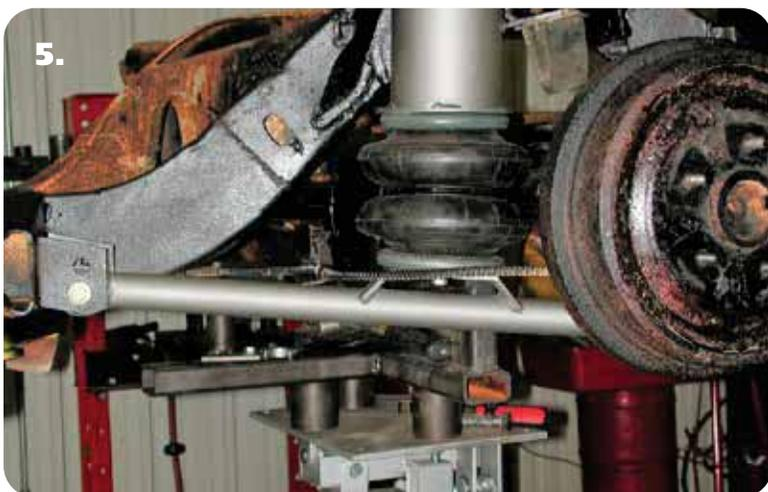
5. Fasten the air spring to the lower StrongArm using a 3/8" x 3/4" bolt, lock washer and flat washer. Torque 15-20 ft-lbs.
