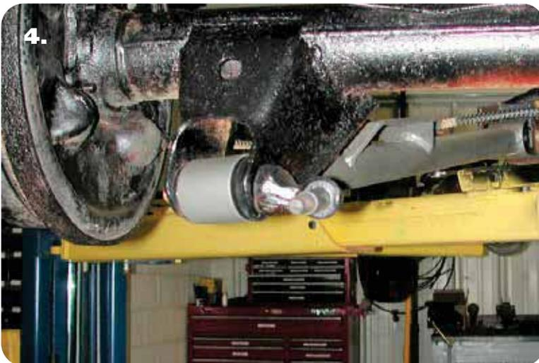
4. The OEM rear bolt will be reused in conjunction with the supplied flat washer and nylok nut. Tighten the bolts/nuts enough to eliminate any gaps.
