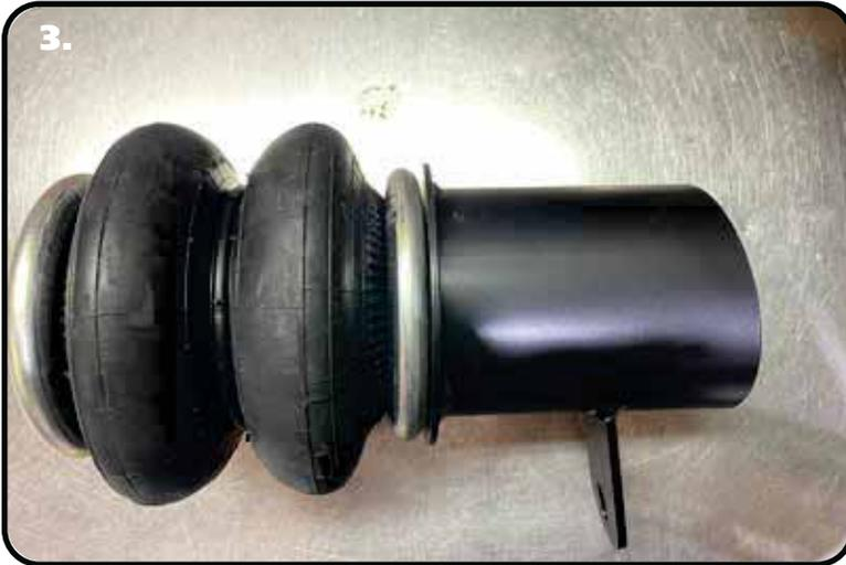
3. Apply thread sealant to the air fitting and screw it into the air spring. Assemble the upper cup bracket to the air spring, using 3/8" - 16 Nylok nuts and 3/8" flat washers. Torque the 3/8" nuts 15-20 ft-lbs.
