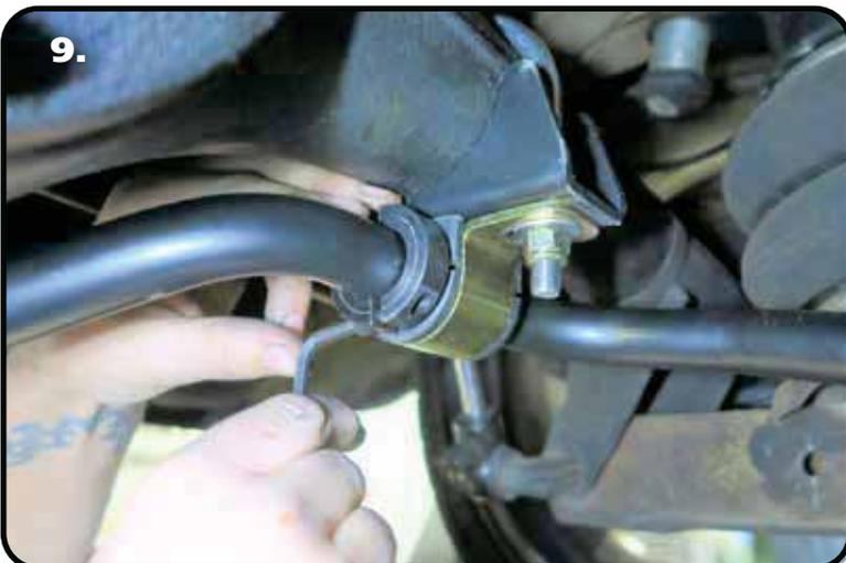
9. Install the locking rings on the outside of each bushing assembly. Use a hex key to take the locking ring apart. Reassemble it on the bar positioned next to the inside of the bushing assembly. Push the locking ring up against the bushing assembly and tighten.
