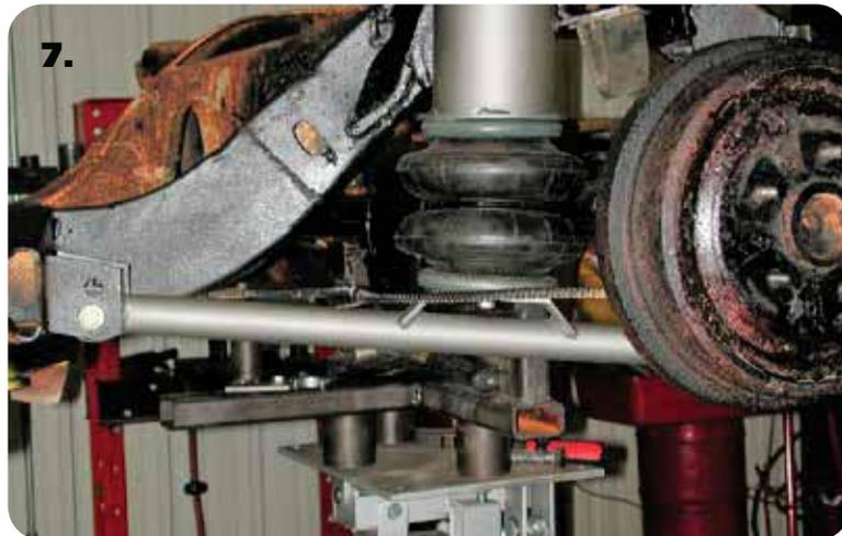
**7.** Fasten the air spring to the lower StrongArm using a 3/8" x 3/4" bolt, lock washer and flat washer. Torque 15-20 ft-lbs.
