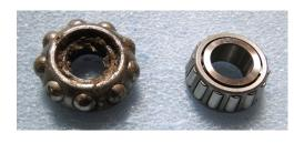
factory ball bearing style on the left with the new tapered roller bearing on the right.
