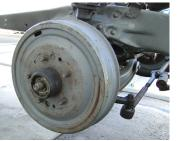
loosen the brake shoes from the drum. This would be a good time to inspect your front brake system. Check for worn pads or leaky wheel cylinders.
