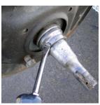
Next, remove the factory iron hub from the brake drum. Original drums are riveted together and you will need to grind the rivets to separate the hub from the brake drum.
