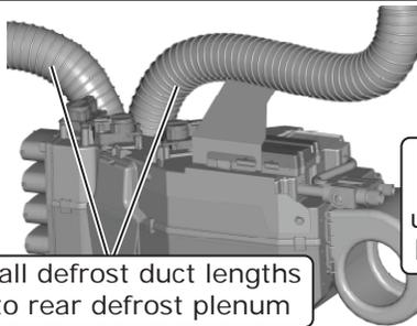
Install defrost duct lengths onto rear defrost plenum
