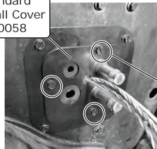
Secure firewall cover using (3) #14 x 3/4" washer head screws
