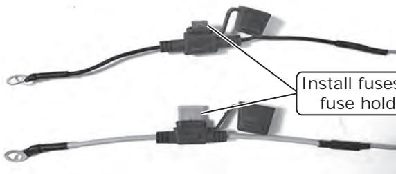
Install fuses into fuse holders
