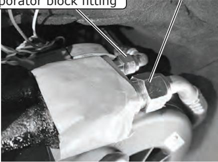
Connect #10 A/C hose to evaporator block fitting
