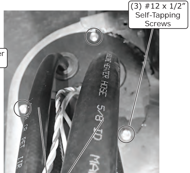
Route A/C and heater hoses through fresh air cover
