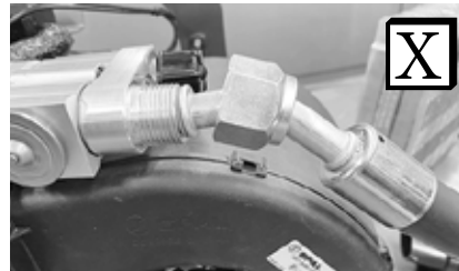
Improperly Seated O-ring Land
